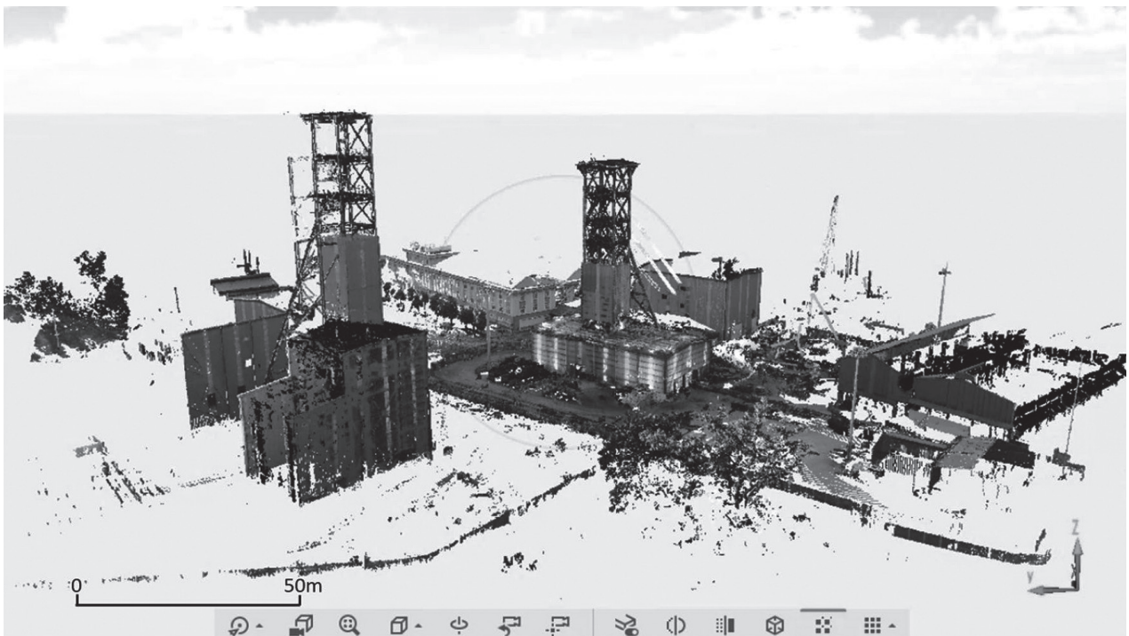
Fig. 1. TLS point cloud displayed in SCENE software [30]
